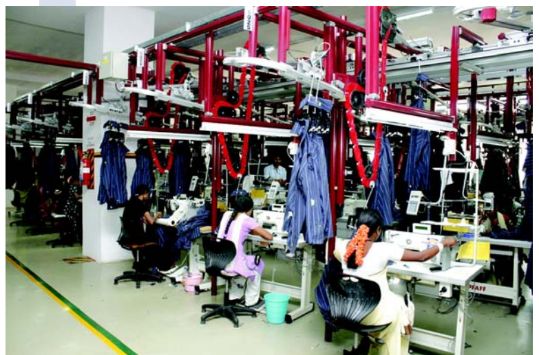
A bundle system (above) requires more Work in Progress than a modular or a UPS system.
