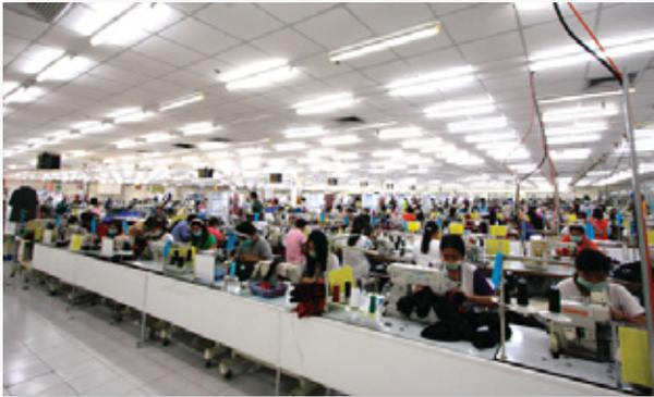
*We have been able to successfully apply PULL system principles so we can then manage material supply to match the plan and also better control WIP thru the many pre sewing operations like embroidery, bonding and screen printing.*
